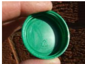
Type 2 milk carton top—off the same bottle as above but marked HDPE! Beware—some milk bottle tops are Type 5, PP
